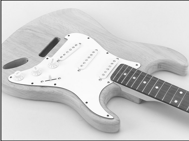
Figure 17. Pick guard alignment.
