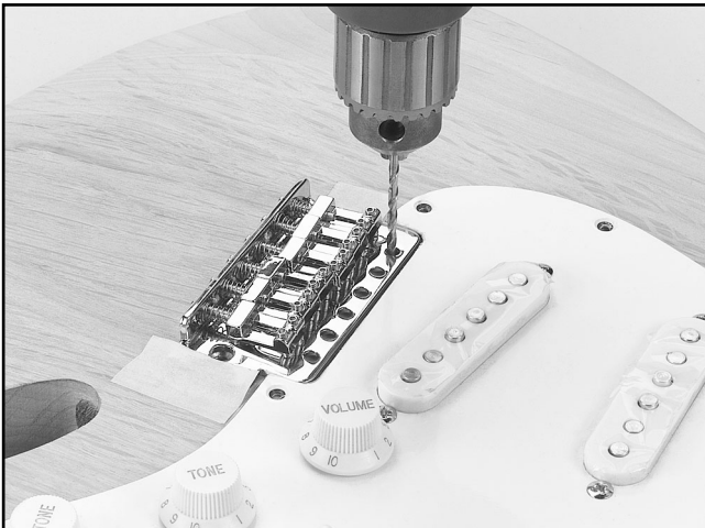
Figure 21. Drilling the bridge mounting holes.
