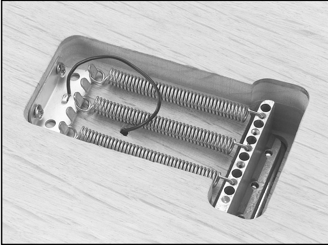
Figure 24. Correct spring placement.
