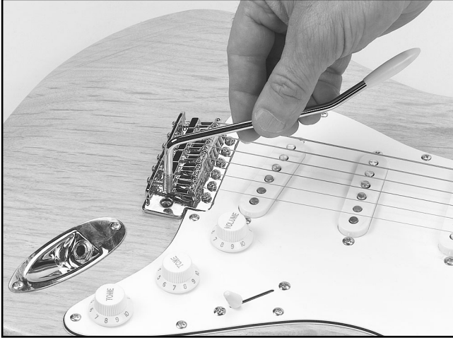
Figure 36. Installing the tremolo arm.
